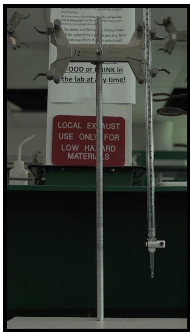
Figure 1.16 Burette with white attachment, called a stopcock. A stopcock controls the flow of the liquid. When positioned vertically, as shown, the stopcock is open, which allows the liquid to drain. [credit: Florida Atlantic University Center for Online and Continuing Education.]
