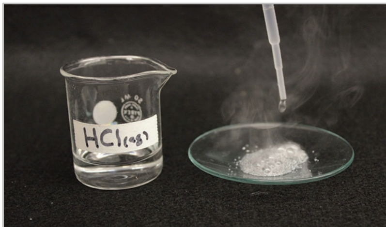
Figure 9.16 The reaction of iron with an acid produces hydrogen. Here, iron reacts with hydrochloric acid. [credit: Mark Ott, as cited in Chemistry 2e . Figure 18.27 . OpenStax. CC BY .]
